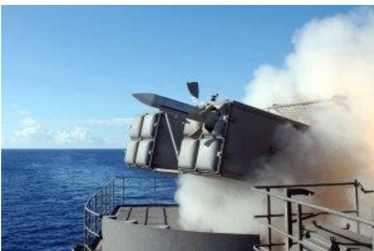
ESSM is an atmospheric, surface-to-air interceptor missile. It is 3.64 m in length and 0.254 m in diameter, with a range of around 50 km. Using solid fuel, ESSM travels at Mach 4, relying on inertial and semi-active radar for guidance. In the Aegis Weapon System variant, an S-band transceiver allows for guidance from the Aegis SPY-1D S-band radar. The missile uses Thrust Vector Control (TVC) to enable tail
